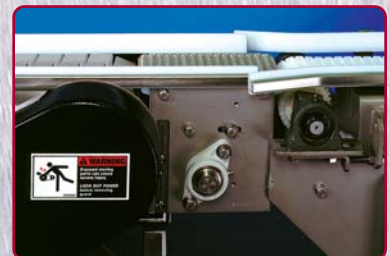
Inline drive-end-to-idle-end transfer.
